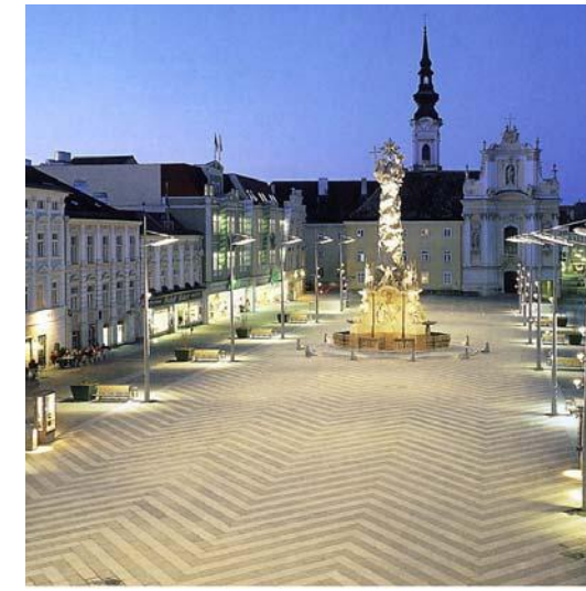
4 Building lighting and the use of LED pavement uplighters demarcate key pedestrian routes, light trees and water
