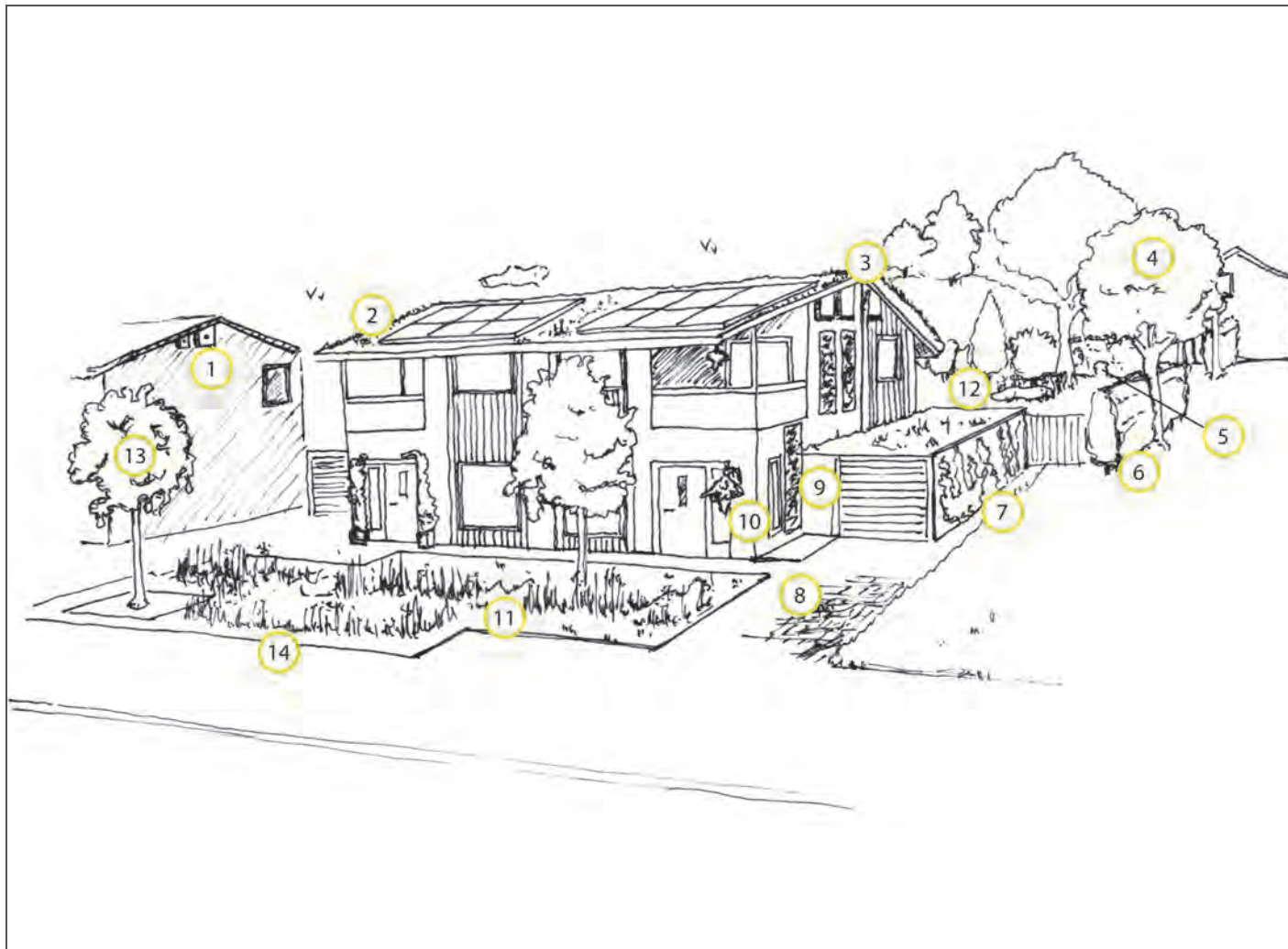
Fig 2.30 Ecological features that can be included on plot as part of the building design to increase biodiversity
